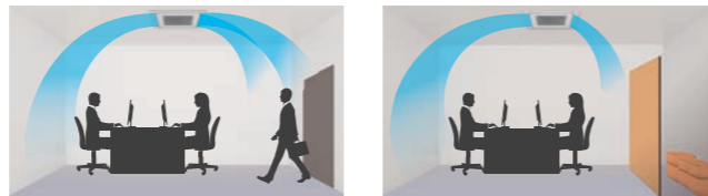
Comfortable air conditioning by preventing direct blowing of cold air and by providing swinging air flow simultaneously.
